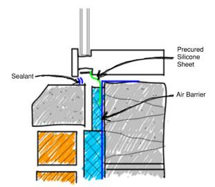
How will the window seal <u>directly</u> to the air barrier at the window's primary seal location? Tip: The example shows a precured silicone sheet that is glazed into the curtainwall – this is a good solution if the primary seal is outboard of the air barrier. If the curtainwall primary seal aligns or is inboard of the air barrier, the precured silicone could be replaced with a sealant joint.
